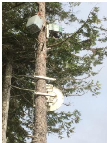
OrcaLab began to experiment with remote cameras in the 1990s and during the NTT Data collaboration was able to show to the world the orcas rubbing from the vantage of two trees above the beach. Step by step, the quality of the video imagery has improved. Prior to 2015, analogue surveillance cameras were used, and in 2016, on the same trees, new higher grade high definition 1080p cameras replaced the 720p cameras Tim had previously installed.
